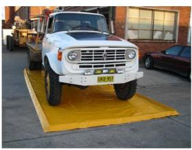
The mat may then be fully erected by unfolding each side completely
