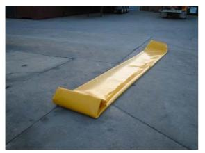
The containment mat is unrolled in the centre of the setup location ensuring that the fold out side is on the centreline of the setup position.
