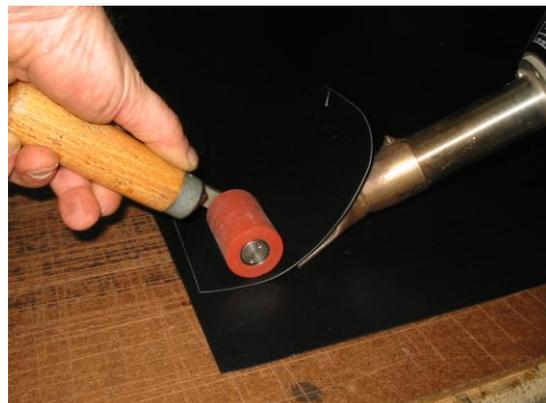
Weld into place using a roller and hot air gun. Note material should be heated until it melts then it is rolled into position.
