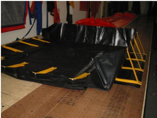
**Step 9:** Where forklifts or other machinery is used to load the bund for smaller units leave two sides down for larger units access may be gained through one end only
