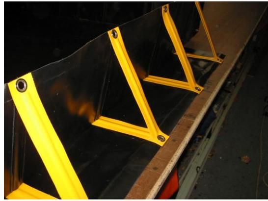
**Step 8:** This process is followed for all supporting legs. NB. grommets on top of legs to secure cover to and grommets on bottom of legs to enable staking to ground
