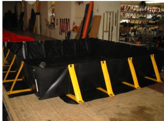
**Step 10:** The remaining sides may be erected. The PBS is now in normal operating configuration
