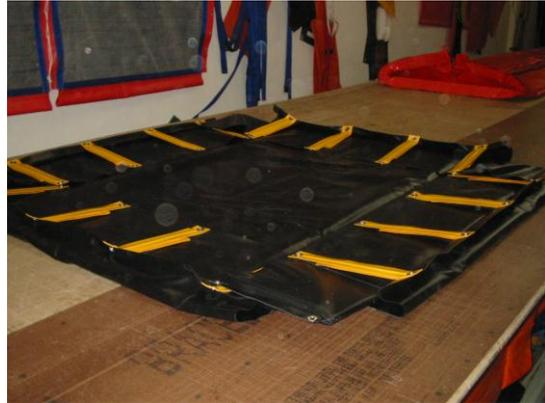
**Step 4:** Depending on the size of the PBS it may be necessary to fold open several times until all sides are exposed
