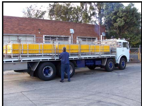
Five racks one high for transport total boom length 500m
