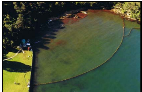
GPF 500 Boom deployed to contain oil against shoreline to facilitate cleanup
