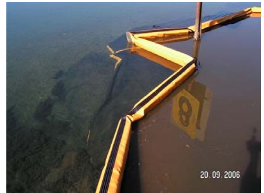
Model SC150TII fitted with a PP8 2m skirt containing heavy sediments in a tidal waterway
